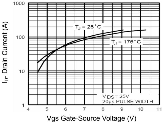
Figure 2 Transfer Characteristics
