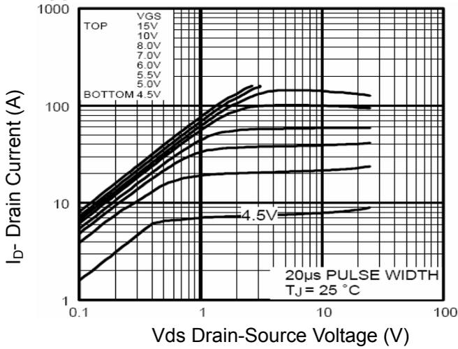
Figure 1 Output Characteristics
